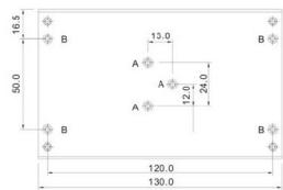
A= For fixture to chassis only A=M3x0.5P B=For fixture to pcb/chassis only B=M3x0.5P
